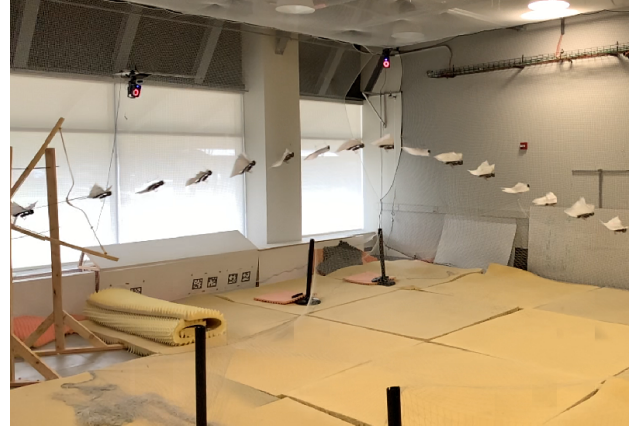
Fig. 6: Open-loop tracking results of 7 flight experiments of the dive maneuver (dark blue for early-phase q_{FL} flights, light blue for late-phase q_{FL} flights) compared with the optimized trajectory (red). The mean of the experiments at each time sample is plotted in solid blue, and the minimum and maximum are plotted in the lighter shadows. The right image displays a single flight result from the early-phase q_{FL} group.
